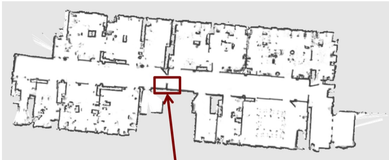
Figure 4.3: A grid map (also called an occupancy grid) is a large gray-scale image, each pixel represents a cell in the physical world. In this picture, cells that are occupied are colored black and empty cells represent free space. A grid map is a useful representation for a robot to localize in this house using observations from its sensors and comparing those to the map.
