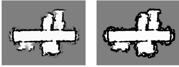
Figure 4.5: (Left) A typical occupancy grid created using a sonar sensor by updating the log-odds-ratio l(m_i | x_{1:k}, y_{1:k}) for all cells i for multiple time-steps k . At the end of the map building process, if l(m_i | x_{1:k}, y_{1:k}) > 0 for a particular cell, we set its occupancy to 1 and to zero otherwise, to get the maximum-likelihood estimate of the occupancy grid on the right.
