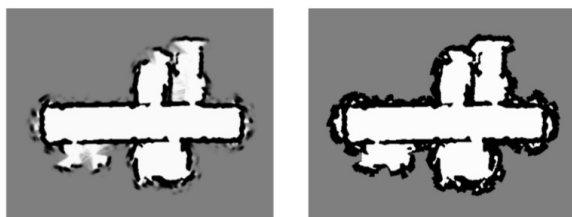
Figure 4.5: (Left) A typical occupancy grid created using a sonar sensor by updating the log-odds-ratio l(m_i \mid x_{1:k}, y_{1:k}) for all cells i for multiple time-steps k . At the end of the map building process, if l(m_i \mid x_{1:k}, y_{1:k}) > 0 for a particular cell, we set its occupancy to 1 and to zero otherwise, to get the maximum-likelihood estimate of the occupancy grid on the right.
